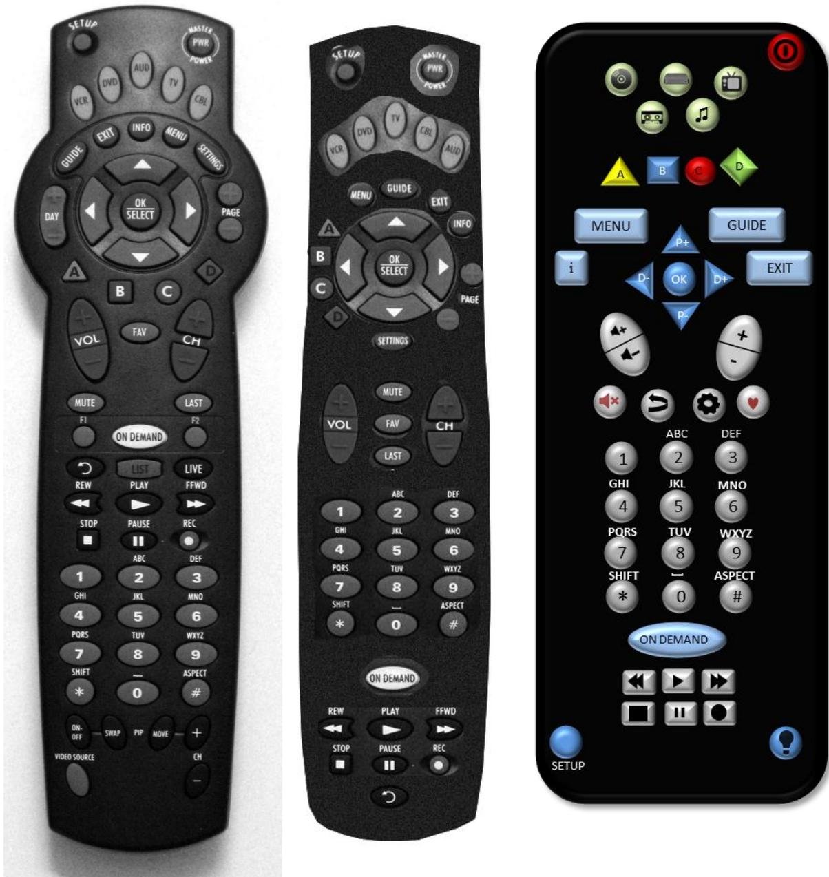
Figure 1. Original, First Redesign, & Iterative Redesign of the Remote Controller
